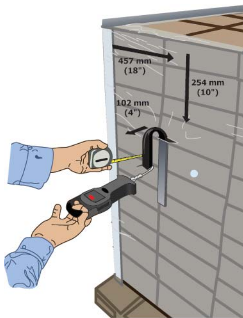
FIG. 5 Pull-Bar Positioning Following Recommended Procedures (see 15.3.2)
