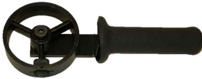
FIG. 1 Marking Wheel Used for Determining Percent Applied Stretch (see 11.2.1)
