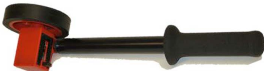
FIG. 2 Tapeless Measure for Evaluating Total Percent Stretch (see 11.2.2)
