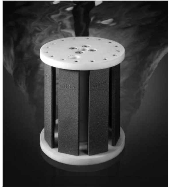
FIG. 2 Photo of Rotating Cage Containing Coupons
