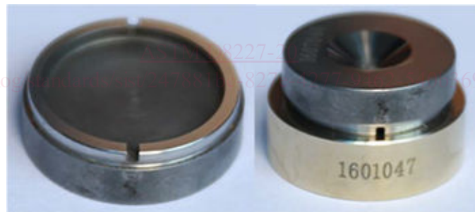
FIG. 3 Contact Surface of Upper Specimen with Slits
