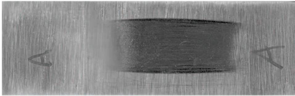
FIG. 5 Typical Uniform Wear Scar
