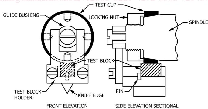
FIG. 3 Assembly of Tester Showing Test Pieces
