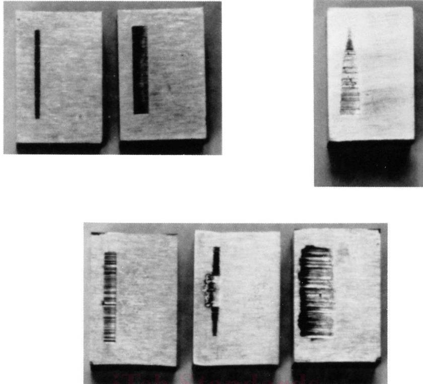
FIG. 1 Test Blocks Showing Various Types of Scar
