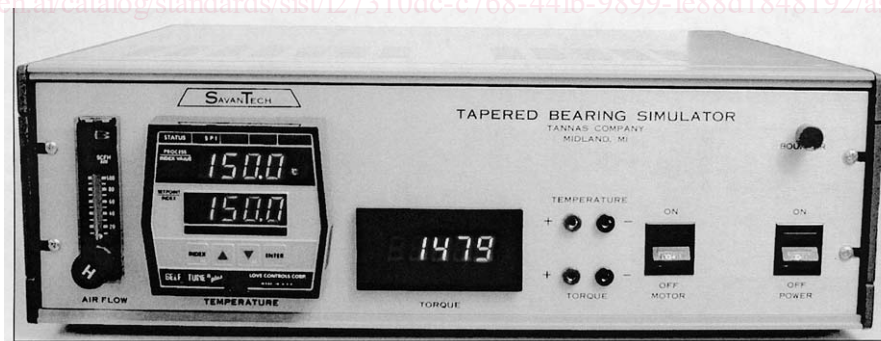
FIG. 4 Control Console for Tapered Bearing Simulator Viscometer Models 400, 500, and 600
