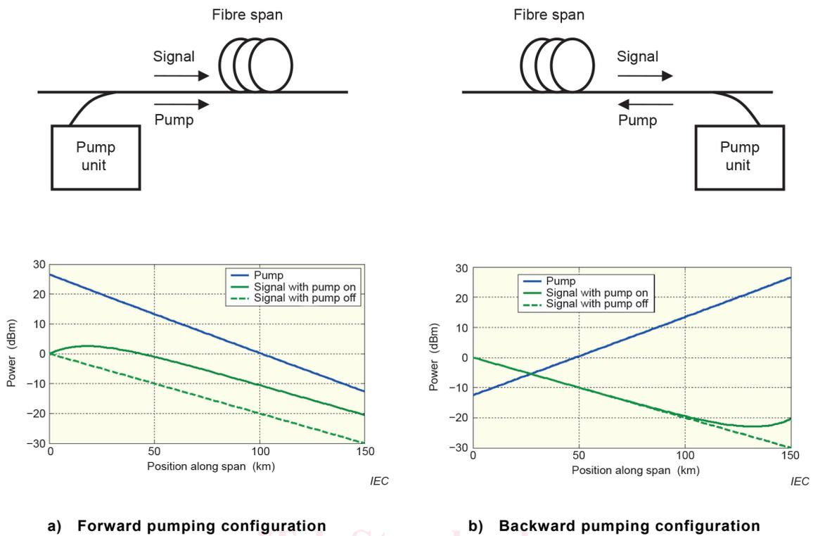
NOTE Two pumps at different wavelengths provide a total of 500 mW, resulting in 10 dB on-off gain across the C-band.
