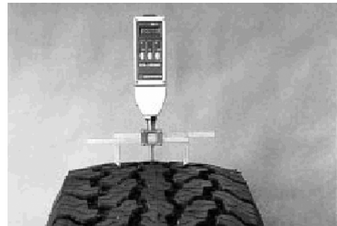
FIG. 5 Measuring the Tread Radius Using the Three-Point Drop
