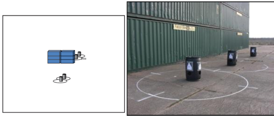
Left: The non-line-of-sight range test method uses an airstrip or flat, paved road with robot test stations placed in front of and behind a wall constructed of stacked 12 m (40 ft) International Standards Organization (ISO) shipping containers. Right: Robot test stations are prototyped behind the wall with targets on the barrels for visual inspection tasks and circular paths for maneuvering tasks.
