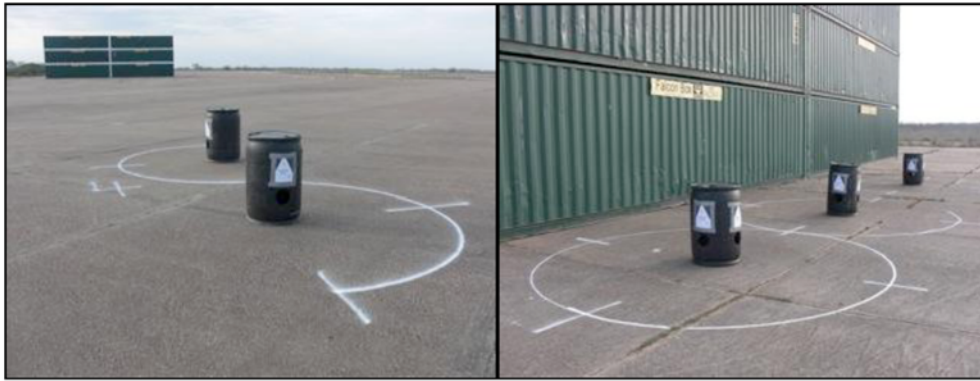
A) The non-line-of-sight range test apparatus includes a reference line-of-sight robot test station 100 m (330 ft) in front of the stacked ISO container obstruction. B) Two additional such test stations are located behind the obstruction to provide non-line-of-sight tasks to perform (one target barrel placed away from the obstruction is not shown).
