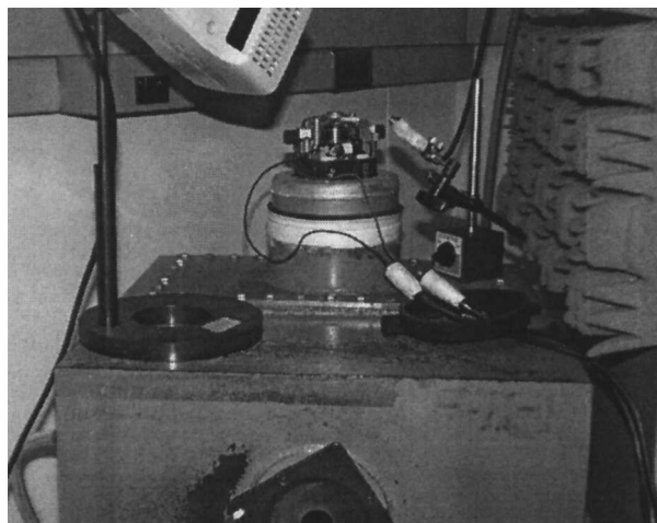
FIG. 1 Motor Mounted to Plenum Chamber
