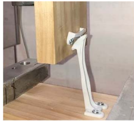
FIG. 3 Example of Failure due to Disengagement
