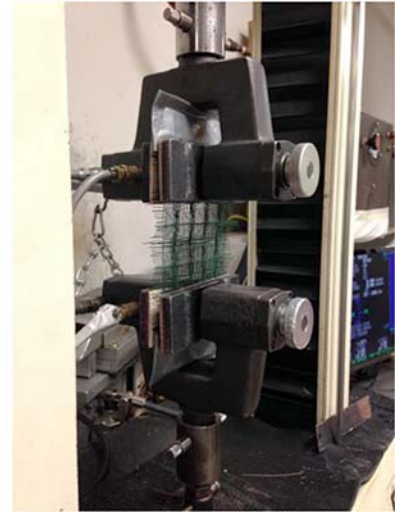
Taped Specimen in Clamps
