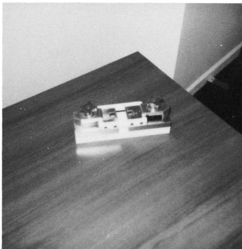
FIG. 3 Cell For Surface Resistance Assembly Photo
