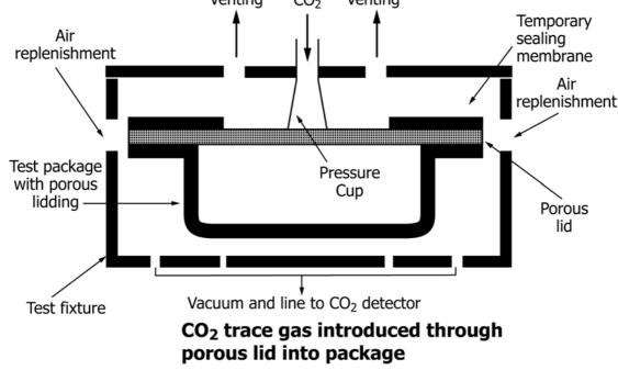
FIG. 1 Schematic of Test Fixture and Test Package
