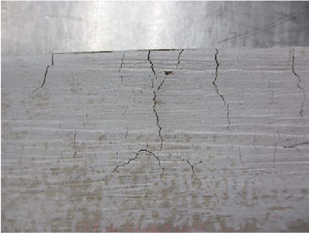
FIG. 11 Crack, Liquid Contamination in Greenware (continued)
