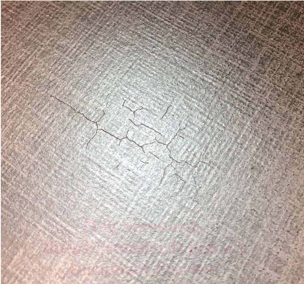
FIG. 11 Crack, Liquid Contaminaton in Greenware
