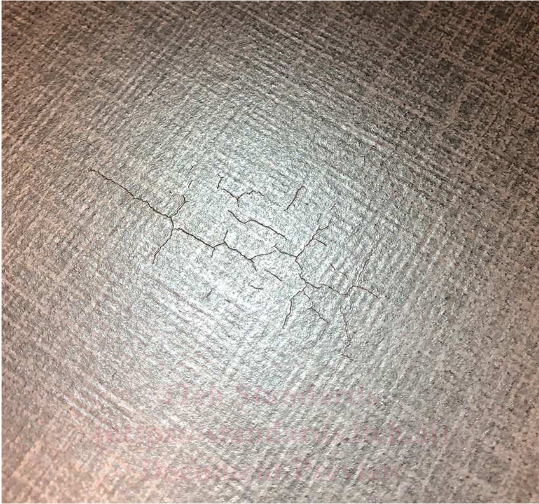
FIG. 11 Crack, Liquid Contaminaon in Greenware
