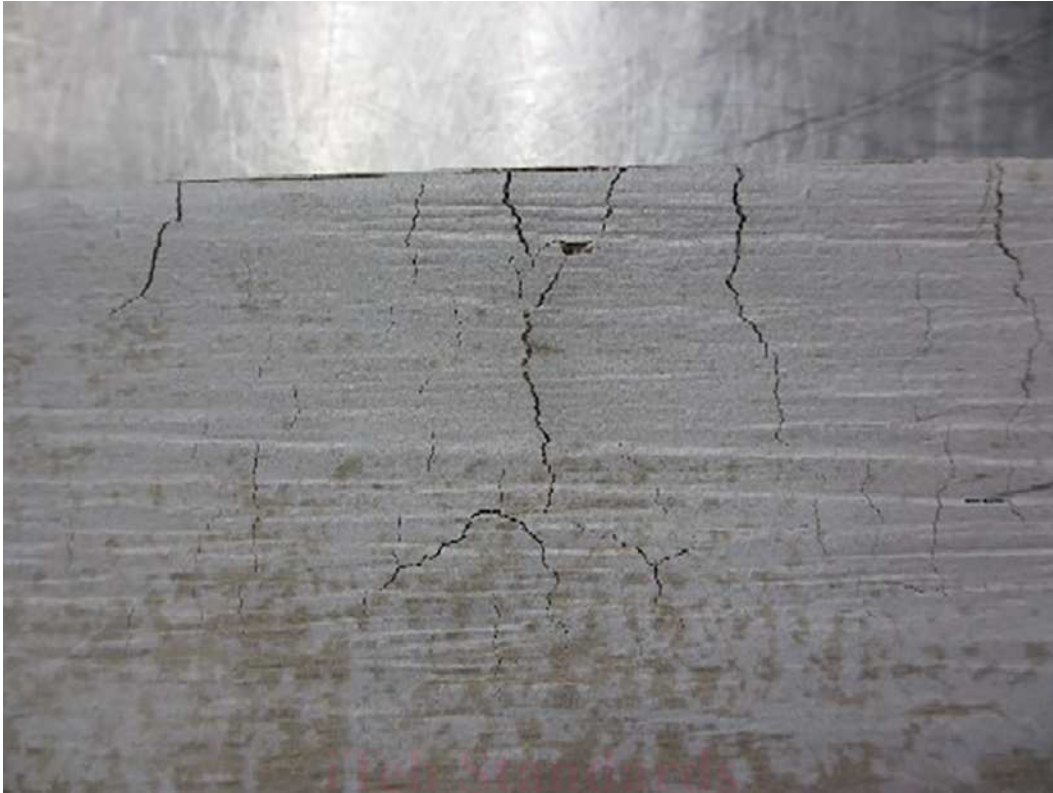
FIG. 11 Crack, Liquid Contamination in Greenware (continued)
