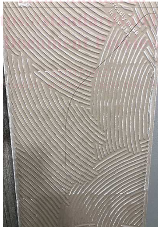
FIG. 9 Crack, (Cooling) Dunting
