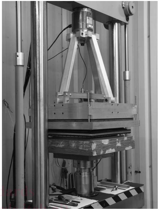
FIG. 3 Two-Dimensional Plate Flexural Test Apparatus
