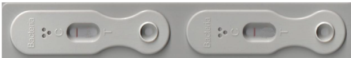
FIG. 5 Bacteria LFD Detecting >750 µg Antigen/L Fuel Phase or >166 µg Antigen/mL Aqueous Phase: No Test Lines Visible
