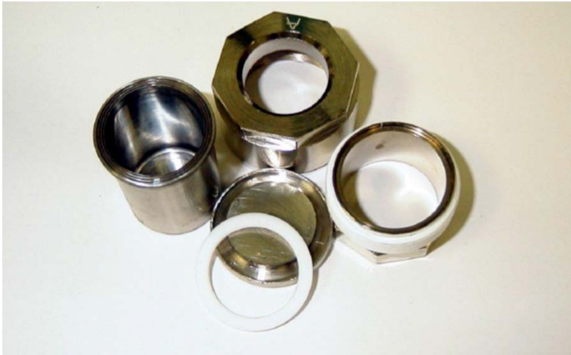
FIG. 1 (a) Desensitized Type 304L Stainless Steel, 22 mL; PCT Vessel and Lid; White Polytetrafluoroethylene Gasket Which Seals Vessel and Lid When Assembly is Closed and Tightened; and Nickel-Plated Brass, Nut, and Screw Vessel Tightening Assembly
