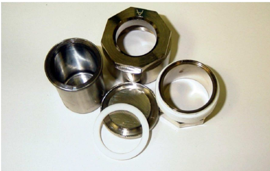
FIG. 1 (a) The (a) Desensitized Type 304L Stainless Steel, 22 mL; PCT Vessel and Lid; a White Polytetrafluoroethylene Gasket Which Seals the Vessel and Lid When the Assembly is Closed and Tightened; and the Nickel-Plated Brass, Nut, and Screw Vessel Tightening Assembly.
