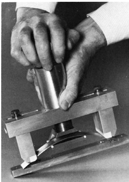
FIG. 2 Stressing Jig and Two-Point Loaded Specimen with Holder (approximately ¼ actual size)
