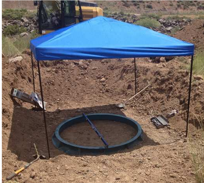
FIG. 1 A 6-ft [1.8-m] Diameter Metal Ring for Determining In-Place Density
