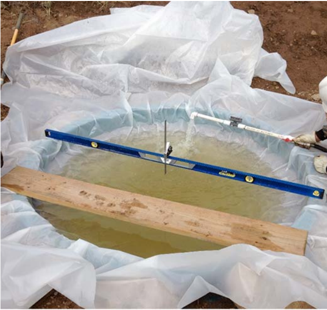
FIG. 3 Measuring the Water-Level Reference with a Carpenter's Square
