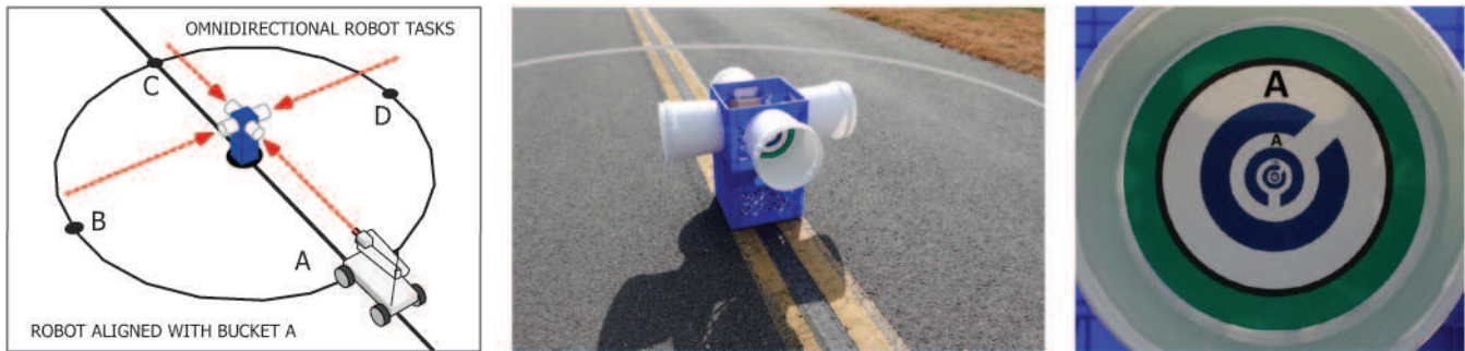
Left) The robot maneuvering tasks include a circular robot path with 3 m [10 ft] radius for the robot to straddle and follow. Middle) The center buckets are perpendicular and limit the viewing angles of the interior targets. Right) Each bucket target has an inscribed ring (shown as green) to evaluate successful alignment along with five increasingly small concentric ring gap orientations to evaluate visual acuity.
