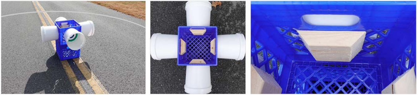
Left) The elevation of the buckets needs to align with various size robots, so some vertical adjustment is necessary. Middle) Stackable crates provide excellent perpendicular mounting surfaces and easy adjustment of elevation. Right) Wood blocks inside the crates enable the buckets to be affixed to the outside surfaces with screws. Bolts, washers, and wingnuts through the bucket and crate can also be used to enable quick set up and stowing.
