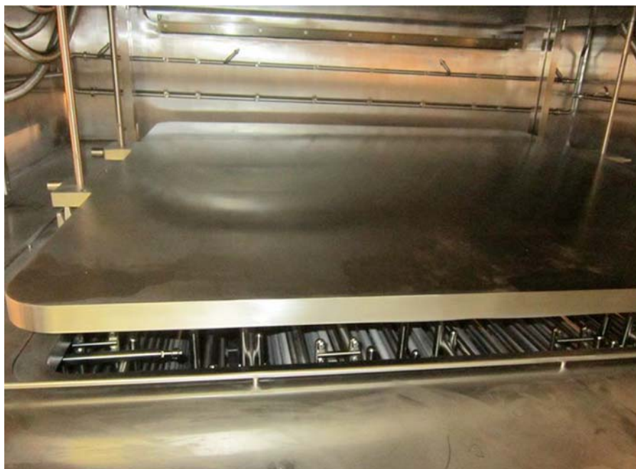
FIG. 7 In This Freeze Dryer, the Condenser is Located below the Chamber Separated by a Hydraulically Actuated Plate
