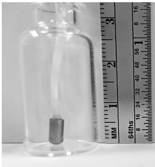
FIG. 4 100 \Omega Platinum RTD Sensor
