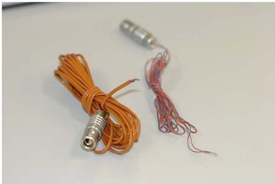
FIG. 3 Thermocouples are Representative of Thermocouples Commonly Used in a Production Environment for Product Temperature Measurement
