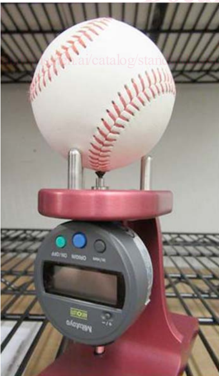
FIG. 3 Example of a Dial Indicator, 3-Point Contact Cradle and Base with Ball
