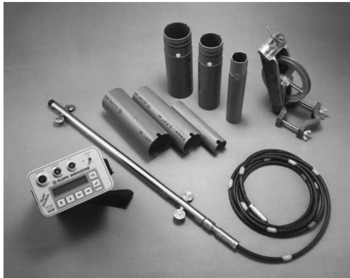
FIG. 1 Typical Components of Method A Inclinometer System
