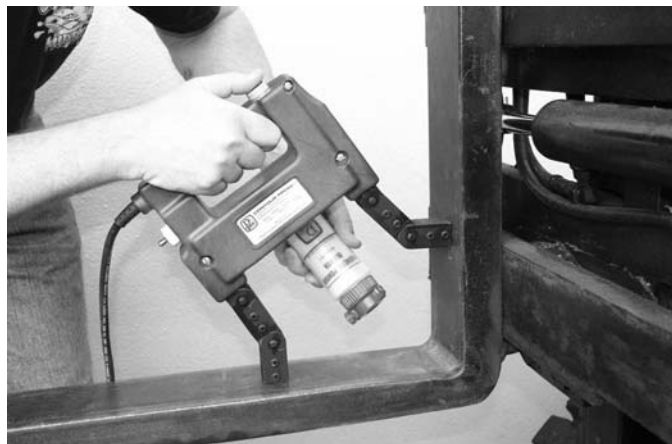
FIG. 1 (a) Articulating Yoke Method of Part Magnetization
