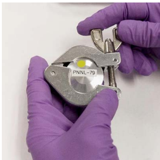
FIG. 2 Fully Assembled SUDA Sampler Including Hinge Clamp
