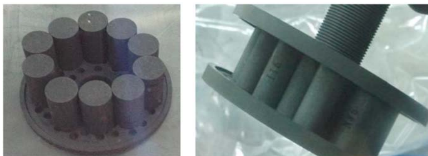
FIG. 2 Sample Holder: Graphite Plates and Sample Rod
