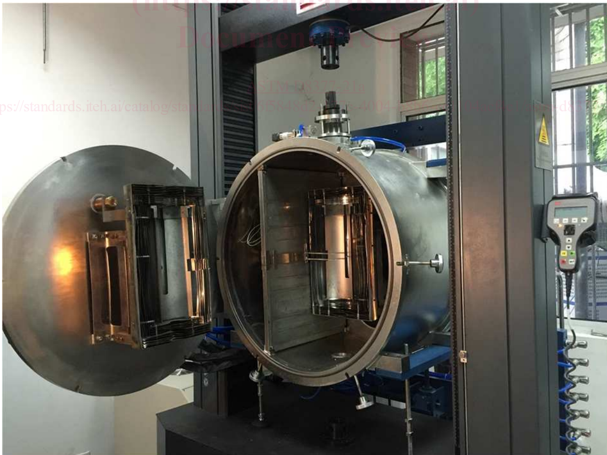
FIG. 1 Overall View of a Representative Testing Compartment and Loading Device
