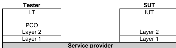
Figure 1: Remote test method
