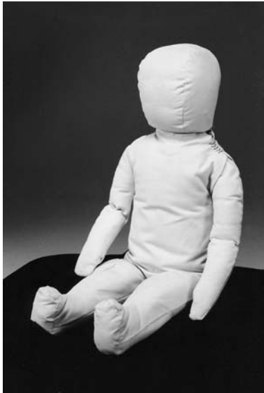
NOTE 1—Department of Transportation, Federal Aviation Administration, Drawing No. SA-1001. FIG. 15 CAMI Dummy, Mark II
