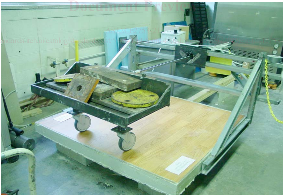
FIG. A1.2 Rolling Load Simulator Prototype
