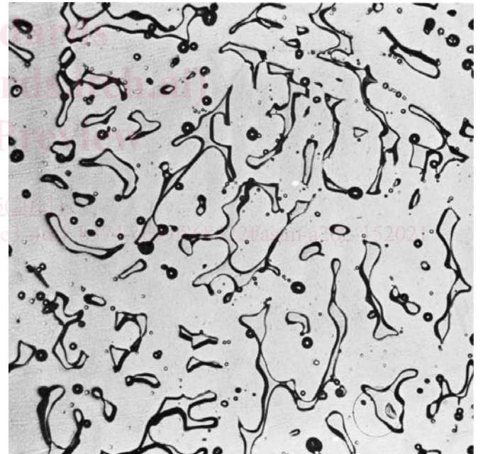
FIG. 4 Isolated Ferrite Pools (250×) (Observed in Castings and Welds. Steps Between Austenite Matrix and Ferrite Pools)
