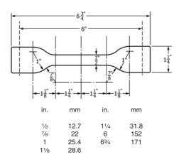
Note 1—The cutting edges shall be beveled on the outside and straight on the inside. The die shall be kept sharp and free of nicks to give clean, even edges on the specimen.
