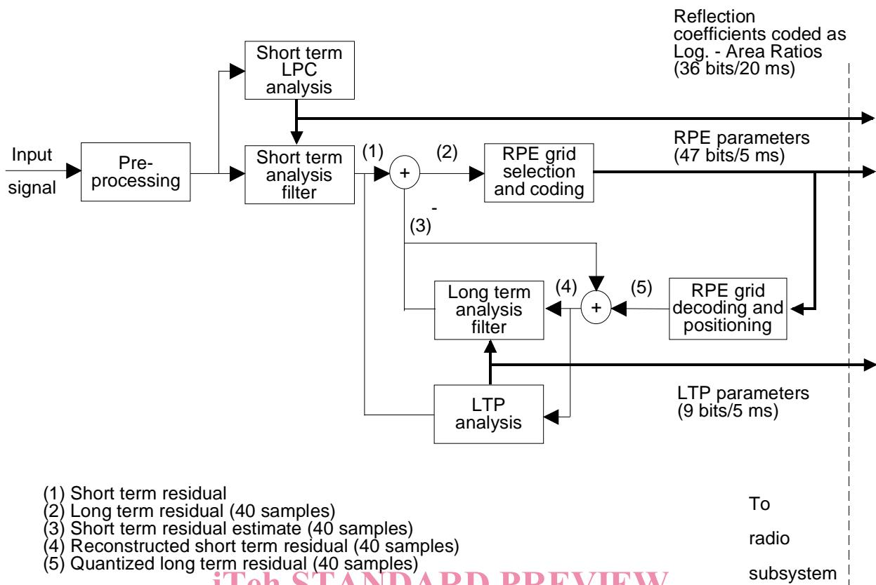
Reflection coefficients coded as Log. - Area Ratios (36 bits/20 ms)
