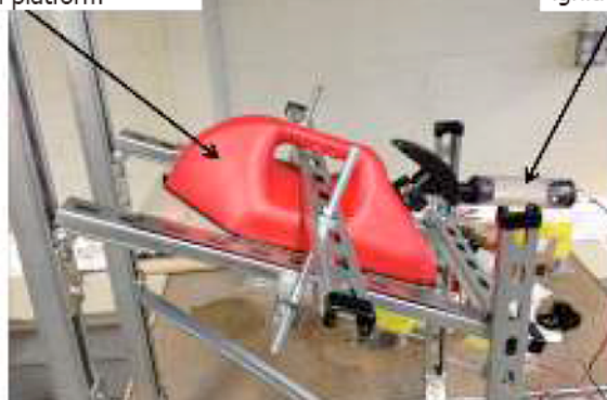
FIG. X1.1 Modified PFC Mounted on Frame and Connected to Ignition Tube
