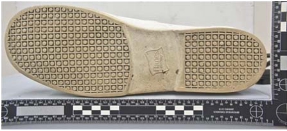
NOTE 1—The most obvious problem is the distortion that can be seen in the straight horizontal part of the ruler that is recorded as being curved. FIG. 1 Photograph of the Bottom of a Shoe (Photographed with a 20 mm Wide Angle Lens on a Full Frame DSLR)
