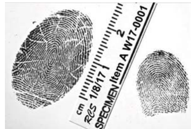
FIG. 7 Filling the Long Dimension of the Viewfinder with the Long Dimension of the Latent Print and Ruler
