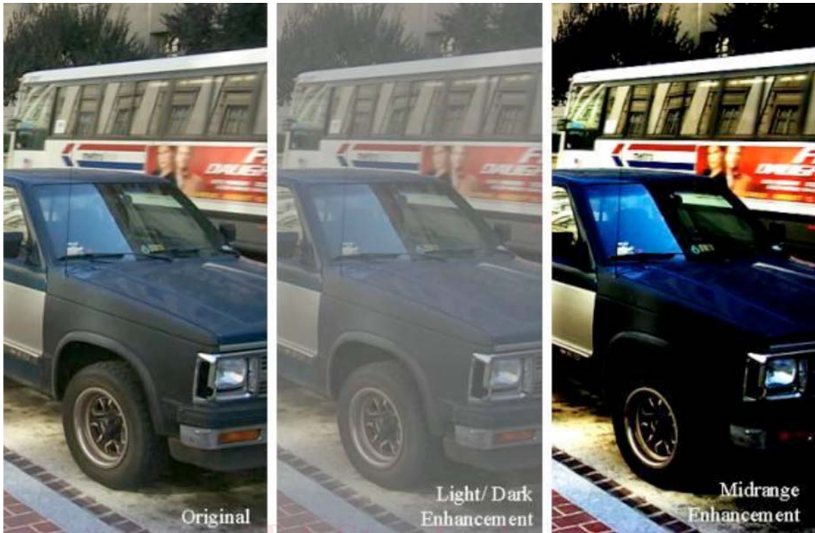
FIG. 2 This Example Shows Nonlinear Contrast Adjustments—Left: Original Image, Middle: Enhancement of Shadow and Highlight Areas at the Expense of Midrange Tones, and Right: Enhancement of Midrange Tones at the Expense of Shadow and Highlight Areas
