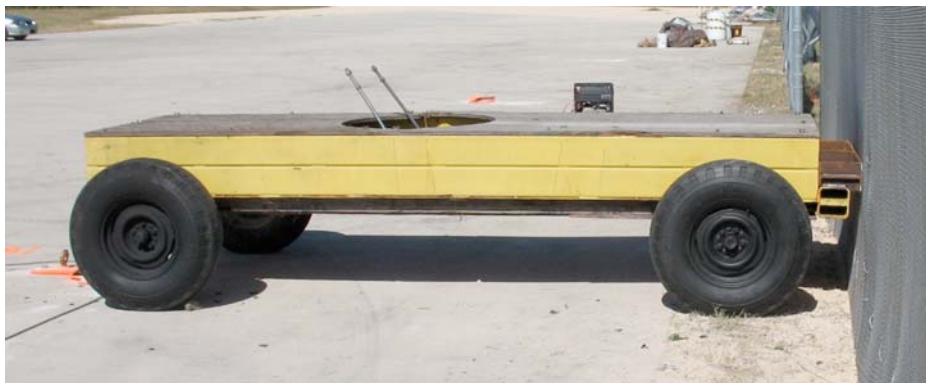
FIG. 1 Bogie Vehicle Used to Simulate an Impact Vehicle
