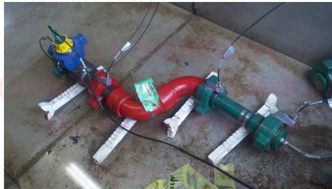
FIG. 2 (b) Sensors 1–4, of a typical non-immersed test A Typical Non-immersed Test (continued)
