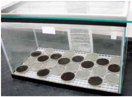
FIG. 2 Typical Environment Chamber Set Up
