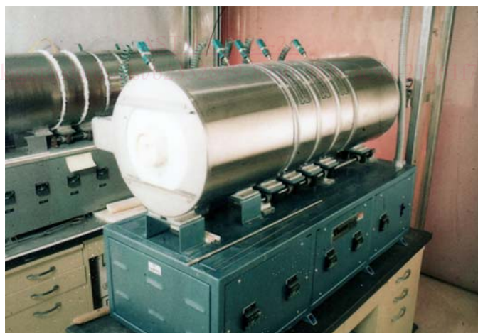
FIG. 3 Photograph of Typical Gradient Temperature Furnace
