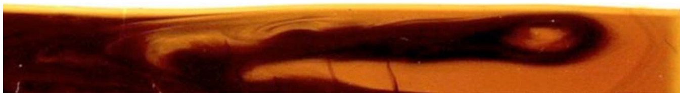
FIG. 7 Crystallization Front in GT Specimen with Convective Flow Patterns
