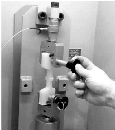
FIG. 5 Pin the Specimen in the Testing Machine
