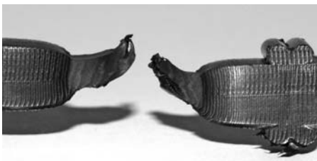
FIG. 2 Ductile Rupture Outside Fusion Interface
