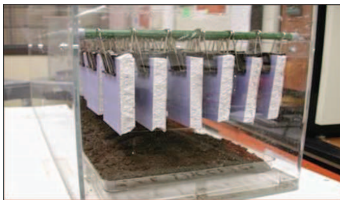
FIG. 1 Environmental-Cabinet Assembly Sample Holding Tank with Test Samples
