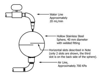
Note 1—Cut three horizontal air slots around circumference of hollow sphere using a 0.20 mm thick diamond lapidary saw covering  $120^{\circ}$  to  $150^{\circ}$  each and spaced approximately 5 mm apart. Air passing through these slots strikes the water (which is flowing over the outer surface of the sphere) to produce a spray.
