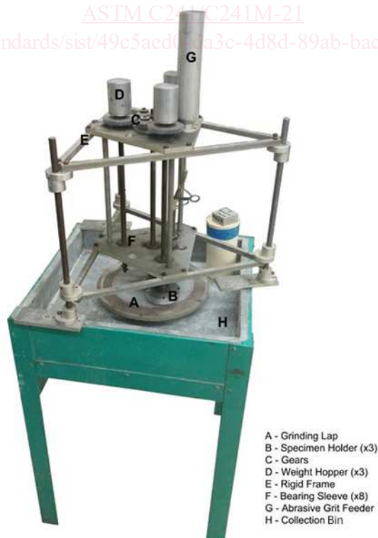
FIG. 1 Apparatus for Abrasion Resistance Test of Stone
