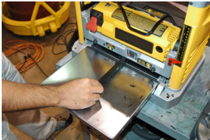
FIG. 7 Electric Planer for Side Bend Specimen Preparation
